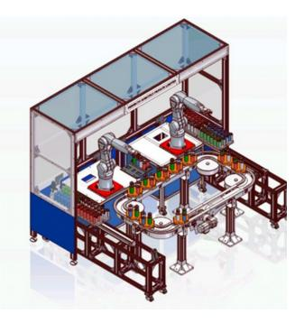
We have developed TIN bottle sorting line for providing the hands-on training which includes all the latest hardware devices with FORD & FCA standards, also it has complex data tracking & Recipe logic. i.e. Stopper Recipe, Infeed Station Scanner, Inspection Station with Machine Vision, Loading/Unloading with Tunnel Lifter, Pre-Stopper, Post-Stopper, Area clear sensor application & many more.
